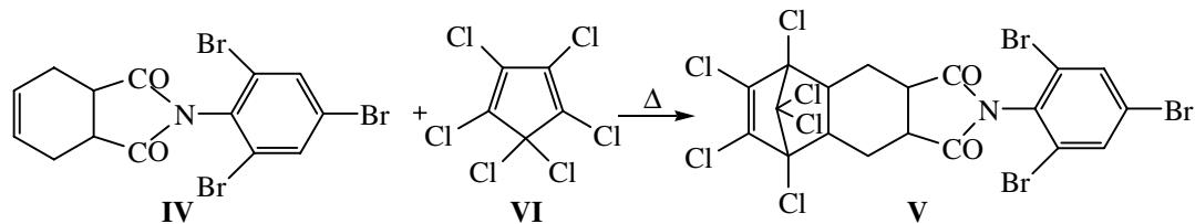
compound **V**. A reaction of *cis*-*N*-2,4,6-tribromophenyl-imide (**IV**) with hexachlorocyclopentadiene (**VI**) at a molar ratio 2:1 and 140°C resulted within 2 h in 99% yield of *endo,exo*-*N*-(2,4,6-tribromophenyl)imide (**V**).
